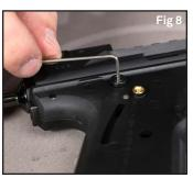
2 Once grips are removed, using a 1/16" hex wrench remove the right side safety lever. (Fig 7)
