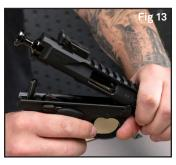
6 Check to make sure that the upper receiver and frame are firmly together and can't be pulled apart.
